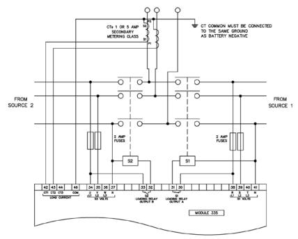
Figure 37 - Typical Wiring Diagram - 2ø 3W (L1-L2)
