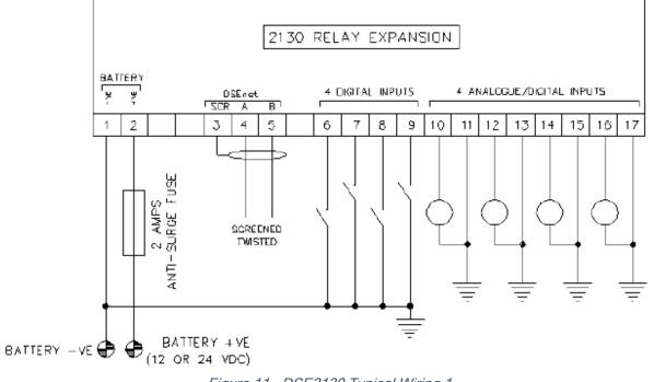
Figure 11 - DSE2130 Typical Wiring 1
