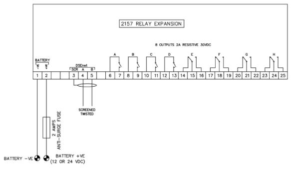
Figure 8 - Expansion Module (Typical) Wiring Diagram
