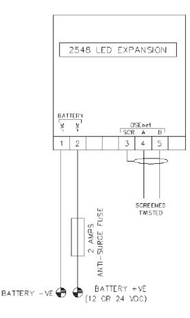
Figure 15 - DSE2548 Typical Wiring
