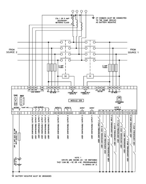
Figure 33 - Example Wiring of the LSE8600 Controller
