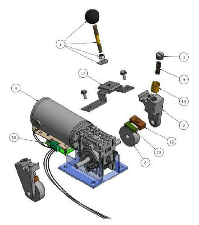
Figure 39 - Gear Motor Assembly
