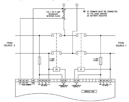
Figure 36 - Typical Wiring Diagram - 1ø 2W
