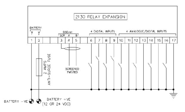
Figure 12 - DSE2130 Typical Wiring 2
