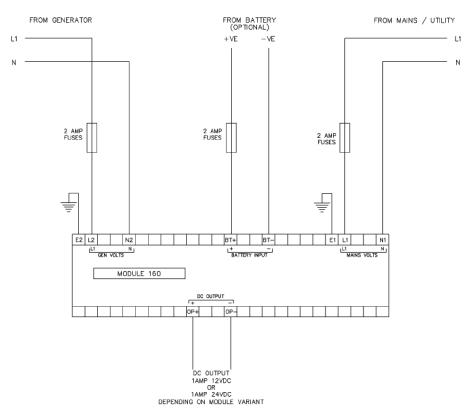
Figure 5 - Self Seeking Power Supply (Typical) Wiring Diagram
