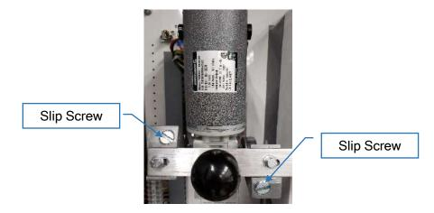
Figure 1 - Motor Slip Screws
