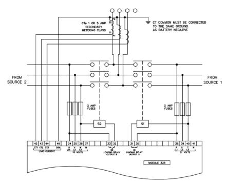
Figure 35 - Typical Wiring Diagram - 3ø 3W
