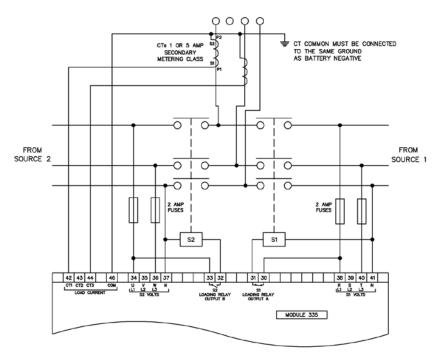
Figure 38 - Typical Wiring Diagram - 2¢ 3W (L1-L3)
