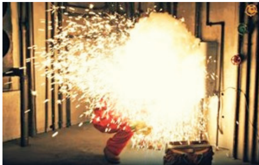
Figure 1 - Arc Flash Example
