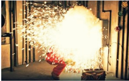
Figure 1 - Arc Flash Example
